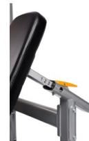
Ankle pad range of motion adjustment lever
