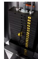
Colour contrasted raised numbering on range of movement adjuster
