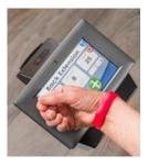
Performance recorder enables maximal isometric force to be measured
